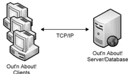
The Out'n About! for Outlook Server is the central point for all client communication and database operations. The server operates as a NT service on Windows NT/2000/XP/2003/Vista/7/8 and includes a service monitor to allow easy configuration and monitoring.
